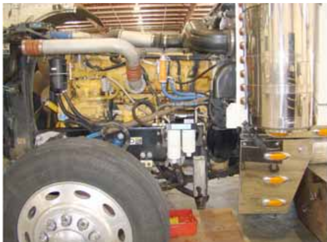
AirDog® mounted on the frame under the steering column to the rear of the shock absorber.
