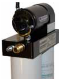
6A-1. Install a straight #10 M JIC x 1/2" M NPT fuel fitting in the AirDog® fuel port marked "ENGINE".
