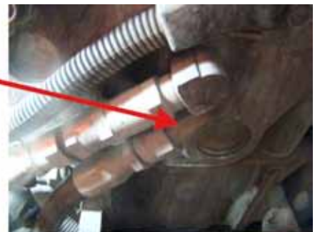
Extended 90° 3/8” NPT x #8 JIC Flare Fitting
