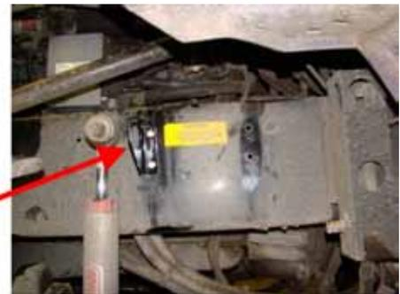
5-2. Mark and center punch the hole locations. Drill a 3/8" hole at each of the 4 locations and attach the AirDog® Champ brackets.
