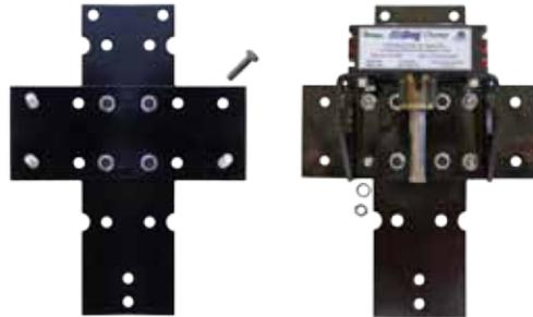
Install 2 of the frame bracket bolts on top of bracket 1 and bracket 3. Slide over frame and install bottom bolt.
