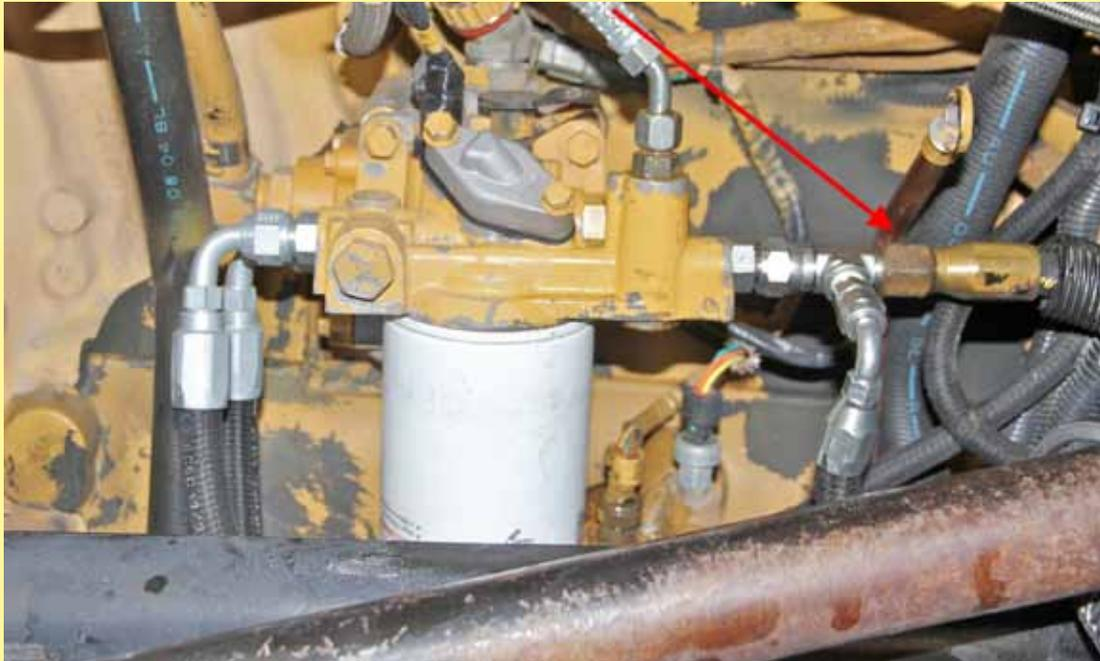
The engine pictured above has a “self priming” AirDog FP-II system installed.
