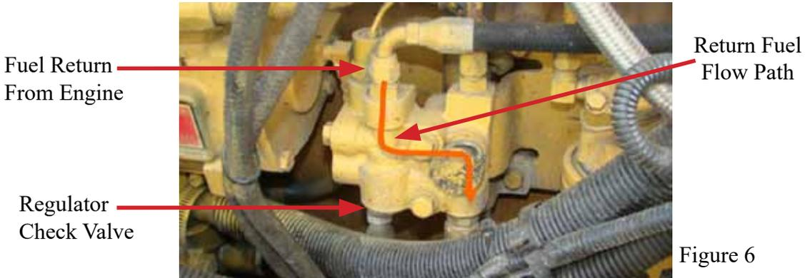
6A-1. Remove the original fuel return line and fitting and install the “Restrictor Fitting” into the fuel return port. (Figure 7)
