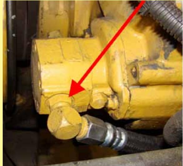
9C-3. Connect the fuel line originally connecting the primary fuel filter to the transfer pump to the AirDog® "Out to Engine" port. If the fuel line is in poor condition or too short to make the connection, replace it with a new fuel line.
