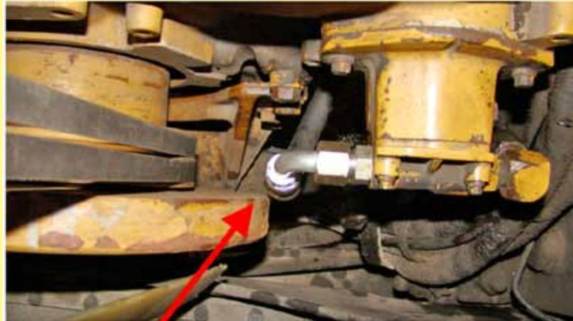
9D-6. Connect the end with the 90° fitting to the transfer pump. DO NOT position the fitting and fuel line too close to the harmonic balancer - see Figure 17. Be sure to have adequate clearance.
