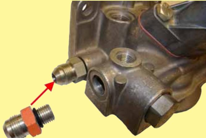
9D-4. Remove the #6 “From Pump” fitting in the secondary filter head and install the #8 M JIC x 3/8 M ORB ported fitting.
