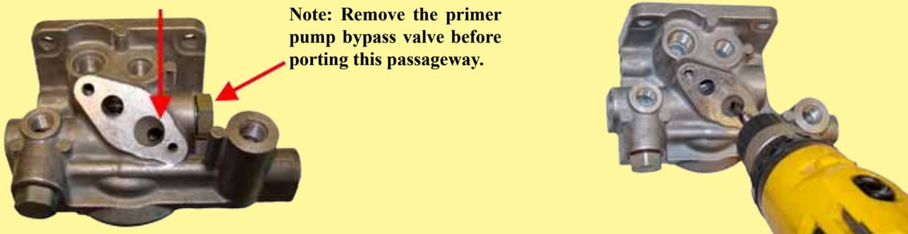
**NOTE:** Be careful not to drill into the fuel filter gasket seat in the underside of the filter head.
