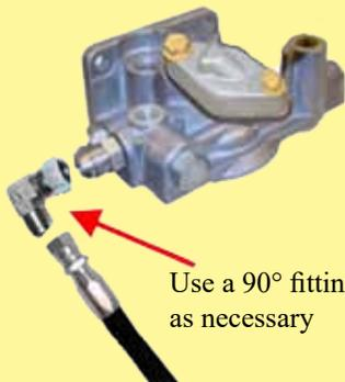
9E-7. Connect the 90° end of the new #8 fuel line to the fitting in the “TO HEAD” port in the secondary fuel filter head.
