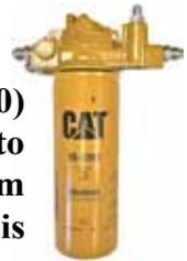
For the CAT 3406E, C10 - C13, C15, C16 and C18 (with filter 1R-0749 or 1R-0750) engine to perform at peak efficiency, the fuel rail pressure must be adequate to completely fill the fuel injectors during the “up” stroke of the plunger. A minimum of 115 PSI to an absolute maximum of no more than 120 PSI at “high idle” is required.
