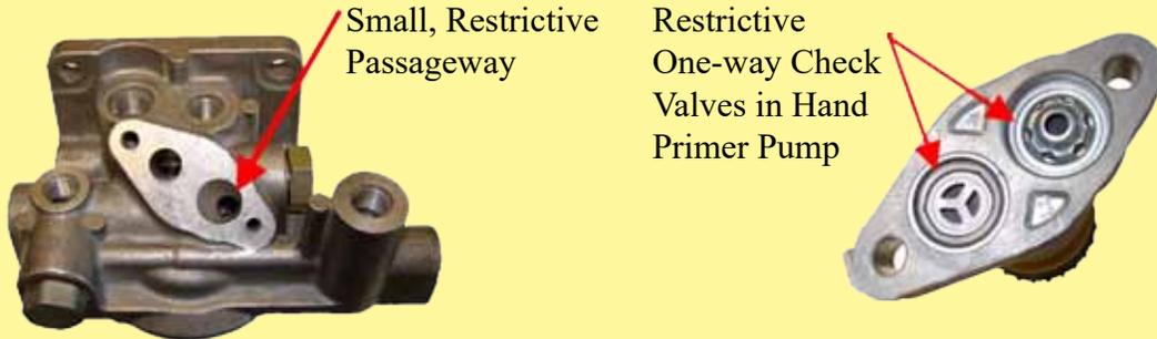
**NOTE:** Perform the following steps to improve fuel flow and engine performance. In most cases, the filter head can be drilled out without removing it from the engine.
