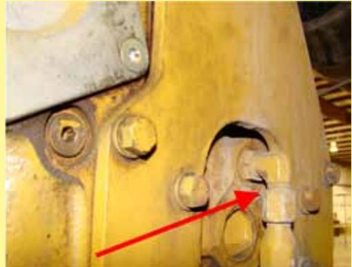
9E-4. Replace the original #6 fitting with a #8 M JIC x 3/8 M ORB ported fitting. You will connect the new fuel line from the secondary fuel filter to the engine head here.
