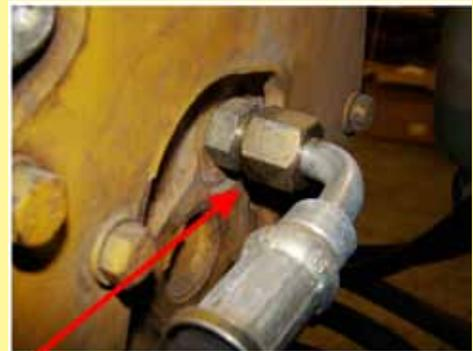
9E-8. Connect the other end of the new #8 fuel line to the ported #8 fitting in the back of the head. Properly tighten all fuel line connections.
