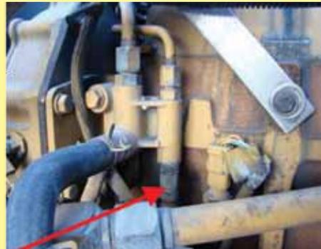
9E-5. Re-route the fuel return line disconnected from the engine in Step 8E-3 and reconnect it where the fuel line to the engine was connected before, as shown above. This reverses the fuel flow through the engine and is only done to make it easier to connect the larger fuel supply line to the back of the engine.
