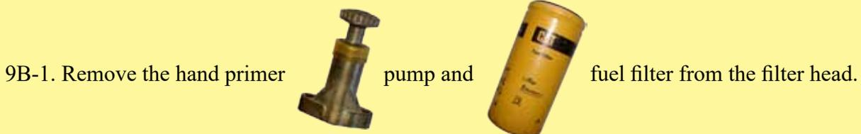
9B-1. Remove the hand primer pump and fuel filter from the filter head.
