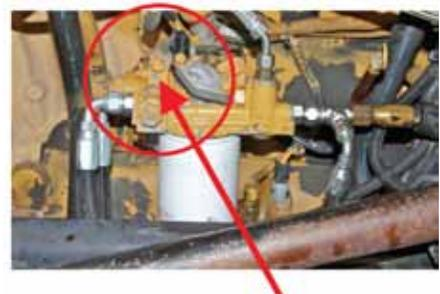
*Connect the Pressure Gauge Here*
