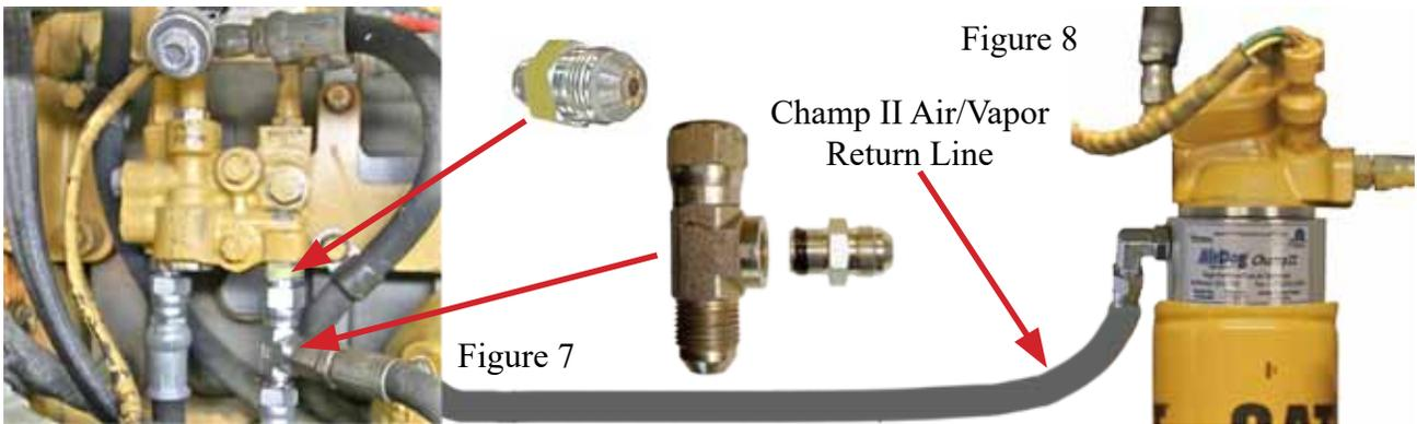
6A-2. Assemble and install the AirDog® Return tee. Reconnect the original fuel return line. (Figure 7)
