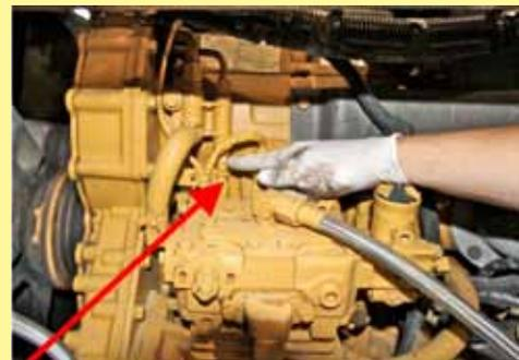
9E-2. Disconnect the other end of the fuel line to the engine and remove the line completely.
