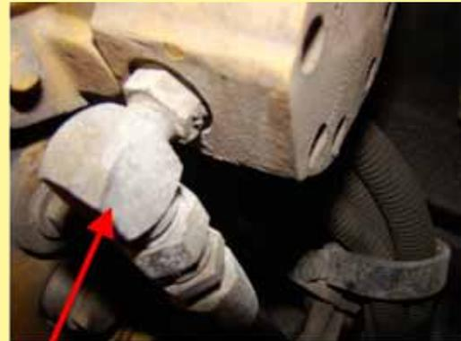
9D-1. Disconnect the fuel line from the discharge side (high pressure side) of the transfer pump.
