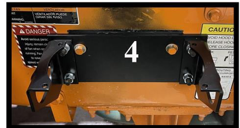
4) Using the original primary filter mounting hardware removed in Step 1, attach the AirDog® BKVM assembly to the truck frame. Tighten securely in place.
