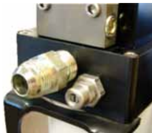
6A-2. Install a straight #10 M JIC x 1/2" M NPT fuel fitting into the fuel inlet port next to the regulator marked "FUEL IN".
