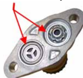
Restrictive One-way Check Valves in Hand Primer Pump
