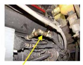
7B-3. Screw the swivel end of the Air/Vapor return Tee onto the engine fuel return fitting. Attach the engine return line to the JIC Male on the other end.
