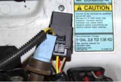
8-2. Route the AirDog® wire harness pump motor lead and the fuel pressure sensor lead to the AirDog® unit. Connect the wire harness pump motor lead (labeled "Attach to Motor") to the AirDog® unit pump motor lead.
