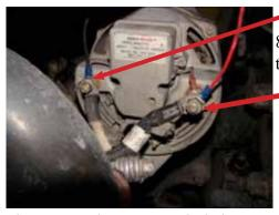
8-12. Connect the red (+) positive lead to the alternator *Hot Lead* going to the battery.
