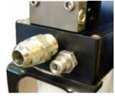
7A-2. Install a straight #10 JIC x ½" NPT fuel fitting into the fuel inlet port next to the pressure regulator marked "FUEL IN".
