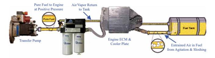
The AirDog® requires only one small return line connected to the engine return line, for quick and easy installations.
