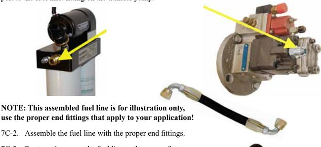
7C-3. Route and connect the fuel line to the proper fitt on the AirDog® and the engine transfer pump. Properly tighten the fittings. Secure the fuel line with zip ties as necessary to prevent abrasion and chaffing.
