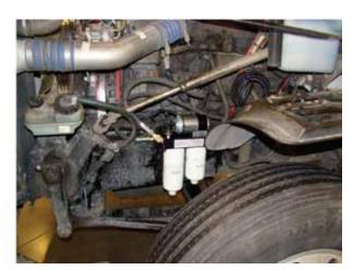
NOTE: When mounting the AirDog® at this location, check for clearance with the tire turned both toward and away from the frame.
