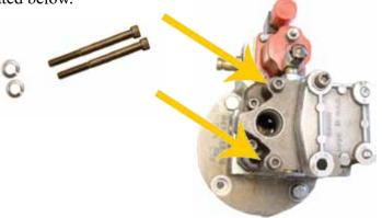
6-3. Install the Pulse Dampener using 2 of the longer ½-20 socket head cap screws and washers previously removed in step 6-1. Be careful to properly install the O-ring in the pulse
