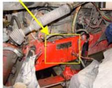
NOTE: Mount the AirDog® as close to the original location of the primary fuel filter as possible. This will allow you, in many cases, to use the original fuel supply line from the fuel tank and also the fuel line to the engine.
