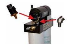
7A-4. Remove the 1/8" NPT plug from the end of the pre-installed 45° fitting in the AirDog® base. Install the pressure sensor into the 45° fitting.
