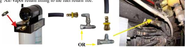
7B-5. Assemble the fuel line using standard procedures for push lock fittings (see page 12). Route and connect the Air/Vapor return line to the air/vapor return fitting on the AirDog® and the return Tee. Properly tighten the fittings. Secure the fuel line with zip ties as necessary to prevent abrasion and chafing.
