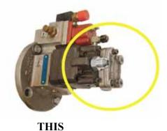
Before connecting the AirDog® to your Cummins N-14 transfer pump, the primary fuel filter assembly mounted on the transfer pump should be removed.
