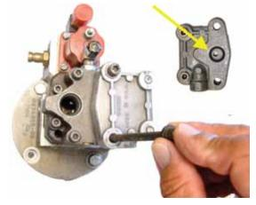
6-4. Install the #10 JIC x 1/2" ORB fuel fitting in the fuel inlet port on the transfer pump. Properly tighten the socket head cap screws and fuel inlet fitting.
