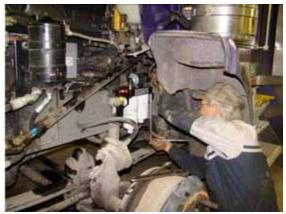
5-7. After mounting the AirDog<sup>®</sup> on the brackets, snug the fasteners to achieve a good relaxed fit. Properly tighten all of the fasteners.
