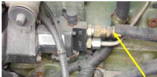
Detroit Diesel Series 60® w/EGR fuel transfer pump fuel Inlet.
