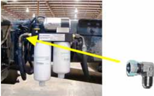
Install a 90° fitting as needed
