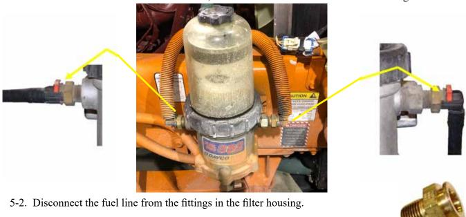
5-3. Should the fuel lines utilize the plastic quick connect fittings as shown, remove the "Quick Connect" fittings from the original fuel filter housing.
