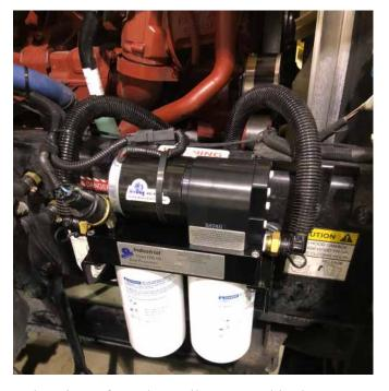
The AirDog® can be easily mounted in the same location as the OE primary fuel filter in this application, as shown in picture.
