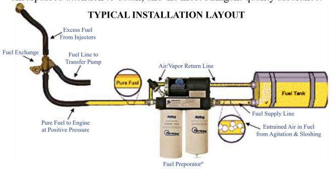
The AirDog® requires only one small return line connected to the engine return line, for quick and easy installations.
