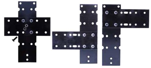
Install 2 of the frame bracket bolts in top of bracket 1 & bracket 3. Slide over frame and install bottom bolt.
