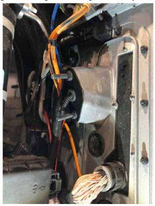
NOTE: Be sure to seal the opening or install a grommet around the wire loom to prevent water leakage and protection from chafing.
