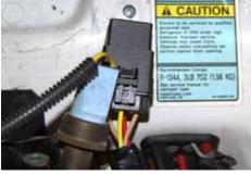
8-2. Route the AirDog® wire harness pump motor lead and the fuel pressure sensor lead to the AirDog® unit. Connect the wire harness pump motor lead (labeled "Attach to Motor") to the AirDog® unit pump motor lead.
