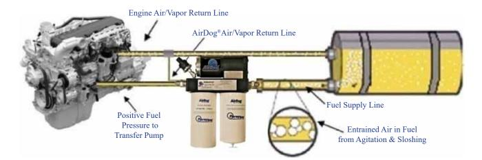
The AirDog<sup>®</sup> requires only one small return line connected to the engine return line, for quick and easy installations.
