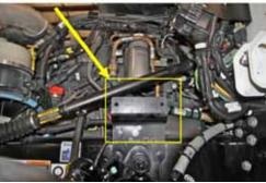
5A-2. For this installation, bolt the Universal Mounting Plate (available from PureFlow<sup>®</sup> Technologies, see page 8) on the original filter bracket.
