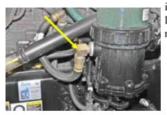
is not in good enough condition or the proper length to make the connection, replace it with a new fuel line.
