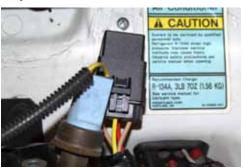
7-2. Route the AirDog<sup>®</sup> wire harness pump motor lead and the fuel pressure sensor lead to the AirDog<sup>®</sup> unit. Connect the wire harness pump motor lead (labeled "Attach to Motor") to the AirDog<sup>®</sup> unit pump motor lead.
