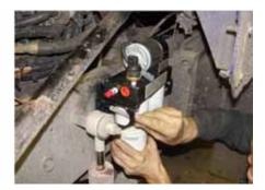
5B-3. While holding the AirDog<sup>®</sup> at the selected mounting location on the frame, mark and center punch each hole location.
