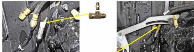
6C-2. Connect the #8 steel braid line (disconnected in 6C-1) to the flare end of the Tee.
