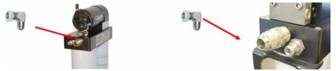
6A-2. Install a straight #10 JIC x  $\frac{1}{2}$ " NPT fuel fitting into the fuel inlet port next to the regulator marked "FUEL IN". Use a 90° swivel fitting as needed when connecting the fuel line.
