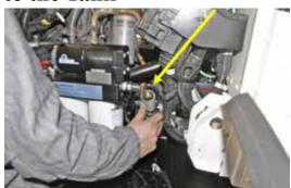
6D. Connect the fuel supply line to the engine that was connected to the original fuel filter to the fitting in the AirDog<sup>®</sup> "Fuel In" port.
