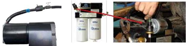
7-3. Connect the AirDog<sup>®</sup> wire harness fuel pressure sensor lead to the AirDog<sup>®</sup> unit fuel pressure sensor.
