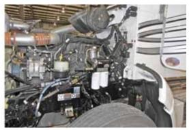
5A-3. Assemble the mounting brackets to the Universal Mounting Plate and then install the AirDog®.
