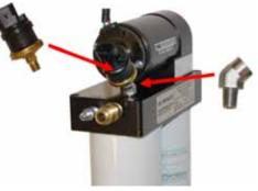
6A-4. Remove the 1/8" NPT plug from the end of the pre-installed 45° fitting in the AirDog<sup>®</sup> base. Install the fuel pressure sensor into the 45° fitting.
