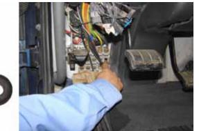
**NOTE:** Be sure to seal the opening or install a grommet around the wire loom to prevent water leakage and protection from chafing.
