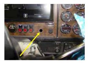
7-8. Drill a 7/16" hole in the dash at the selected location. Be very careful when drilling. Do not damage components located behind the dash. Remove the nut from the indicator light.
