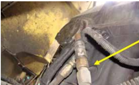
Engine Fuel Return Line
