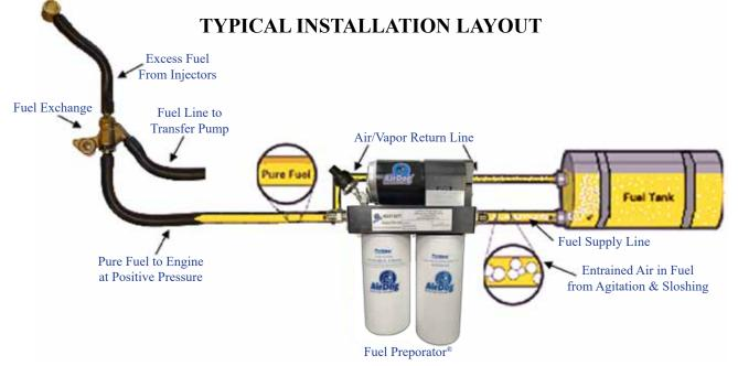
The AirDog<sup>®</sup> requires only one small return line connected to the engine return line, for quick and easy installations.
