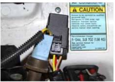
8-2. Route the AirDog<sup>®</sup> wire harness pump motor lead and the fuel pressure sensor lead to the AirDog® unit. Connect the wire harness pump motor lead (labeled "Attach to Motor") to the AirDog<sup>®</sup> unit pump motor lead.
