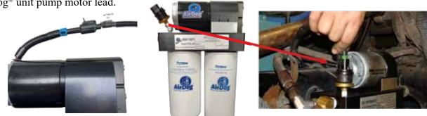
8-3. Connect the AirDog<sup>®</sup> wire harness fuel pressure sensor lead to the AirDog<sup>®</sup> unit fuel pressure sensor.
