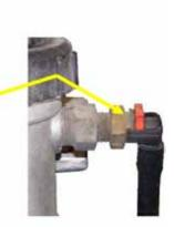
5-2. Disconnect the fuel line from the fittings in the filter housing.
