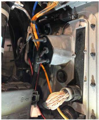
**NOTE:** Be sure to seal the opening or install a grommet around the wire loom to prevent water leakage and protection from chafing.
