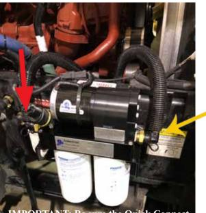
**IMPORTANT:** Be sure the Quick Connect fitting clicks when connecting the fuel line.
