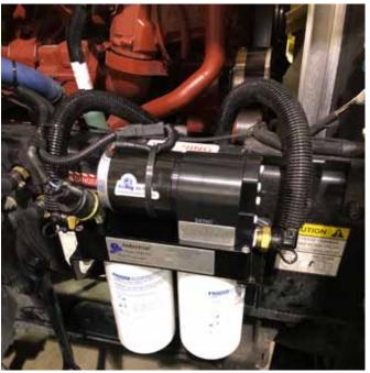
The AirDog<sup>®</sup> can be easily mounted in the same location as the OE primary fuel filter in this application, as shown in picture.
