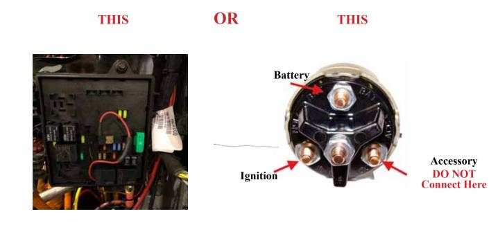
INSTALLING THE AIRDOG<sup>®</sup> WIRE HARNESS INDICATOR LIGHT Amber LED Indicator Light
