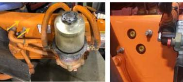
5-5. Remove the original primary filter assembly from the frame.
