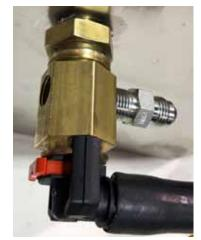
7G-2. Measure and cut the length of #6 fuel line required, when properly routed, to connect the AirDog<sup>®</sup> return line to the quick connect adapter installed in the fuel tank.
