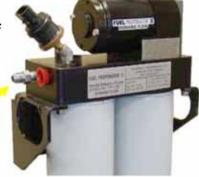
6-3. Install the Quick Connect x <sup>1</sup>/<sub>2</sub> NPT fitting removed from the original primary filter in the port marked **"ENGINE".**
