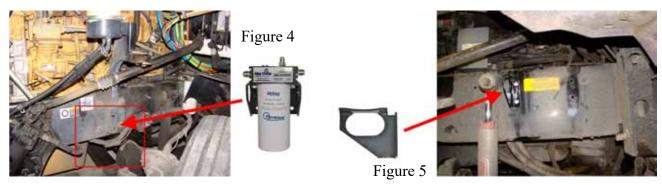
5-2. Mark and center punch the hole locations. Drill a 3/8" hole at each of the 4 locations and attach the AirDog<sup>®</sup> Champ brackets.
