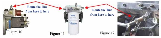
6A-6. Connect a new #6 fuel line to the fuel transfer pump and to the AirDog<sup>®</sup> Champ "FUEL IN" port (Figures 10 & 11).
