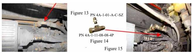
6B-2. Assemble the AirDog<sup>®</sup> Champ return tee (Figure 14) and install it on the engine fuel return fitting. Reconnect the engine return line to the return tee.
