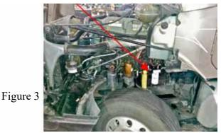
5-1. Hold the AirDog<sup>®</sup> Champ, with the brackets and filter attached, next to the frame at the selected mounting location. Check for clearance. If mounted between the frame and steer tire, turn the steering wheel fully to the left and right to check for tire clearance.
