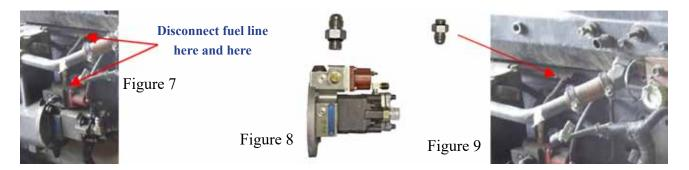
6A-3. Install the # 5 ORB x #6 JIC (PN 4A-1-25-05-06-S) in the fuel solenoid (Fig. 8).
