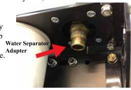
3. Unscrew the lock nut from the fuel heater nipple.
