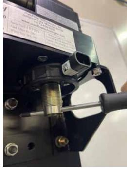
7. Reinstall the Water Separator (or install new), and tighten as normal (hand-tighten + max of <sup>3</sup>/<sub>4</sub> turn with a filter wrench).
