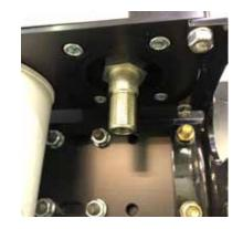
5. Install the 300W Heater Element, o-ring facing upward (toward the AirDog® base) over the fuel heater nipple. Hold in place.
