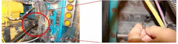
7-5 Route the AirDog® wire harness trigger lead (red wire with no connector/plug) and indicator light lead through the firewall.
