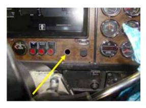
7-8. Drill a 7/16" hole in the dash at the selected location. Be very careful when drilling. Do not damage components located behind the dash. Remove the nut from the indicator light.
