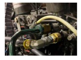
6C-2. Test fit the included 3/8" fuel line between the AirDog® TANK port and fuel return at the Paccar filter housing. If there is extra length in the provided line, carefully cut it to the length required for your installation.
