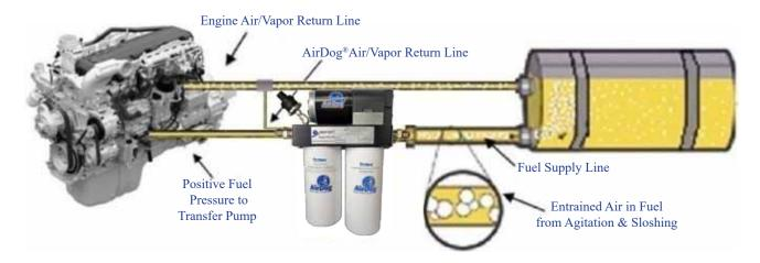
The AirDog® requires only one small return line connected to the engine return line, for quick and easy installations.
