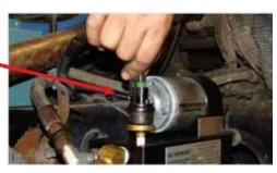
7-3. Connect the AirDog® wire harness fuel pressure sensor lead to the AirDog® unit fuel pressure sensor.
