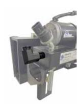
6A-3. Install the AirDog® return fitting (1/4"-NPT x #6 JIC) into the TANK port on the AirDog® base.
