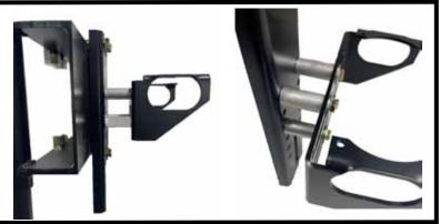
Once the mounting brackets are secured, use the provided 1/4"-20 x 2" socket-head cap screws and appropriately sized split lock washers and hex nuts to loosely assemble the AirDog® onto the 1-piece Bracket. After mounting the AirDog® on the 1-piece Bracket, snug all fasteners to achieve a good relaxed fit.
