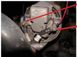
7-12. Connect the red (+) positive lead to the alternator *Hot Lead* going to the battery.
