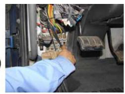
NOTE: Be sure to seal the opening or install a grommet around the wire loom to prevent water leakage and protection from chafing.
