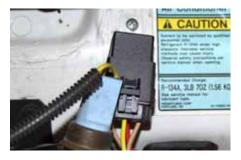
7-2. Route the AirDog® wire harness pump motor lead and the fuel pressure sensor lead to the AirDog® unit. Connect the wire harness pump motor lead (labeled "Attach to Motor") to the AirDog® unit pump motor lead.
