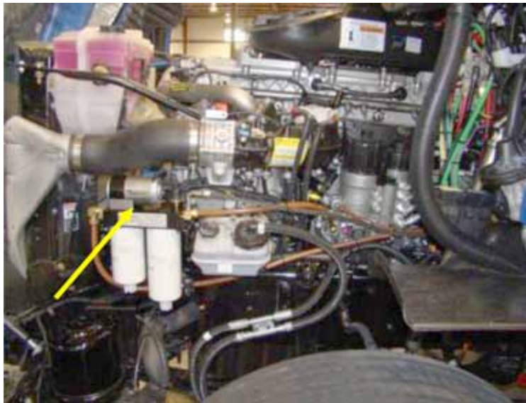
This picture finds space to mount the AirDog® on a bracket in the location of the original primary fuel filter.
