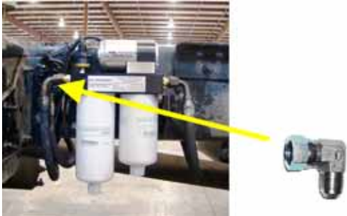
Install a 90° fitting as needed
