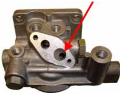
Small, Restrictive Passageway
