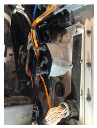
NOTE: Be sure to seal the opening or install a grommet around the wire loom to prevent water leakage and protection from chafing.
