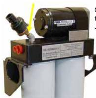
6-1. Remove the 1/8 NPT plug located in the end of the 45° elbow. Install the pressure sensor into the elbow.
