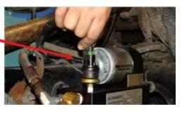
8-3. Connect the AirDog® wire harness fuel pressure sensor lead to the AirDog® unit fuel pressure sensor.
