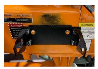
5-6. Loosely assemble the AirDog® to the mounting bracket. Snug the fasteners to achieve a good relaxed fit and then properly torque all the fasteners.
