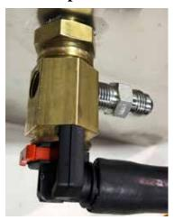
7G-2. Measure and cut the length of #6 fuel line required, when properly routed, to connect the AirDog® return line to the quick connect adapter installed in the fuel tank.
