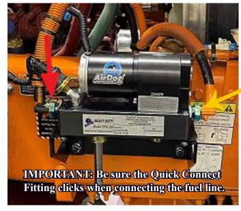
**NOTE**: In cases where extra clearance is required it may be necessary to use provided 1/2 M NPT x 1/2 F NPT 90° Elbow & 1/2 F NPT x #8 F JICX fittings to extend the quick connect port.
