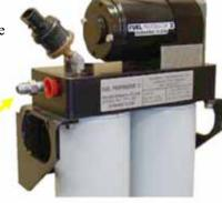
6-3. Install one Quick Connect x 1/2" NPT fitting into the port marked ENGINE.
