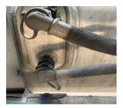
7D-2. Measure and cut provided 1/2 fuel line to length. First, insert #8F JICX x 1/2 Push-Lock Hose Barbs on each end. Next, install one hose end into the AirDog® base marked "FUEL IN". Then connect the other hose end to the quick connect fitting.
