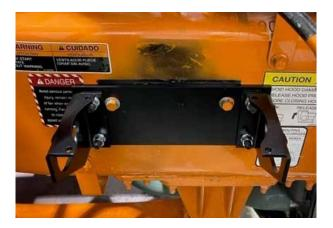
5-6. Loosely assemble the AirDog<sup>®</sup> to the mounting bracket. Snug the fasteners to achieve a good relaxed fit and then properly torque all the fasteners.
