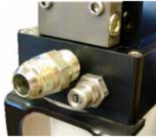
6A-1. Install a straight #10 M JIC x 1/2" M NPT fuel fitting in the AirDog® fuel port marked "ENGINE".
