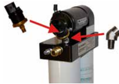
6A-4. Remove the 1/8" NPT plug from the end of the pre-installed 45° fitting in the AirDog® base. Install the pressure sensor into the 45° fitting.
