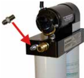
6A-3. Install the #6 M JIC x 1/4" M NPT return fitting into the air/vapor return port marked "TANK".
