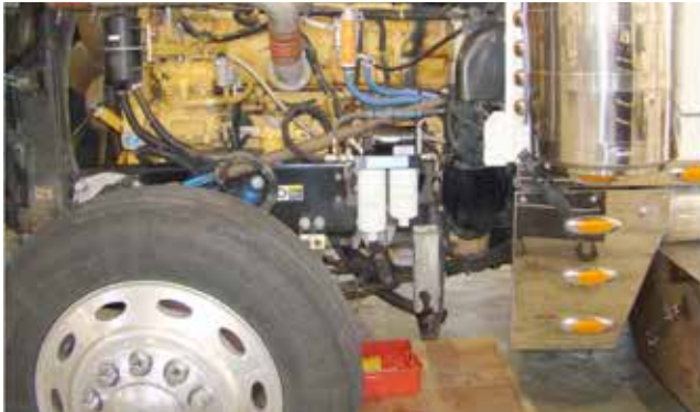
AirDog® mounted on the frame under the steering column to the rear of the shock absorber.
