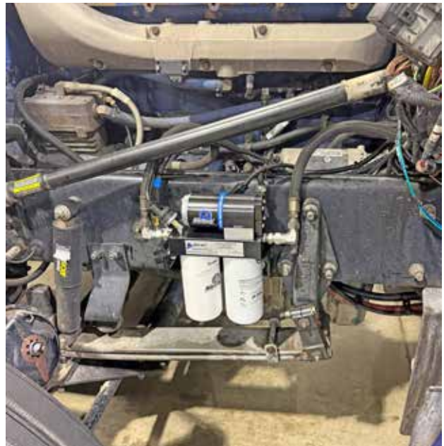
This picture shows how to find space to mount the AirDog® to the rear of the shock absorber.
