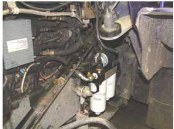
This picture shows how to find space to mount the AirDog® to the rear of the shock absorber.
