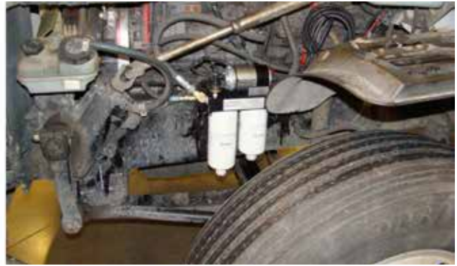
AirDog® mounted under the steering column ahead of the shock absorber.
