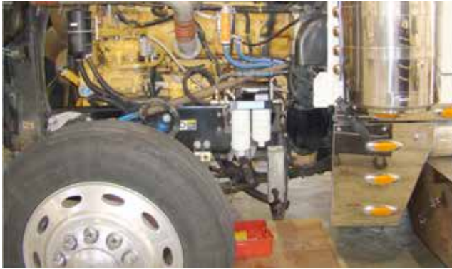
AirDog® mounted on the frame under the steering column to the rear of the shock absorber.
