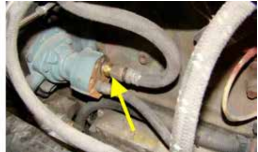
Detroit Diesel Series 60® fuel transfer pump fuel inlet
