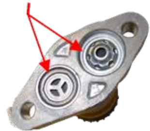
Restrictive One-way Check Valves in Hand Primer Pump
